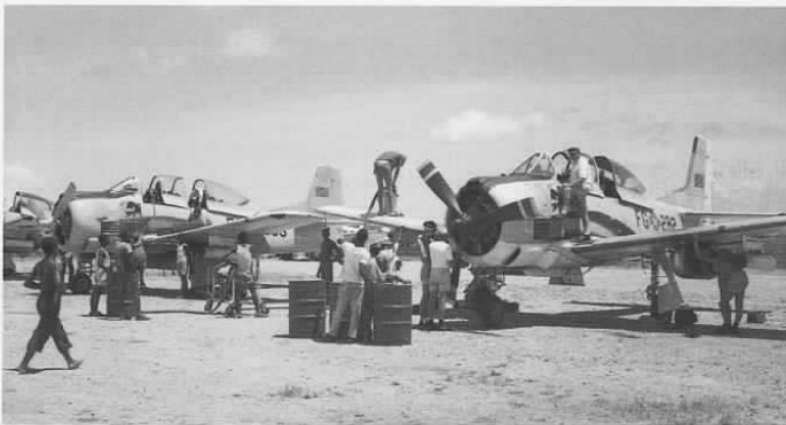
Busy scene at Albertville, with aircraft being rearmed and refueled between missions. Note the large fuel filter used when filling up FG-282. (Lars Carlsson)
