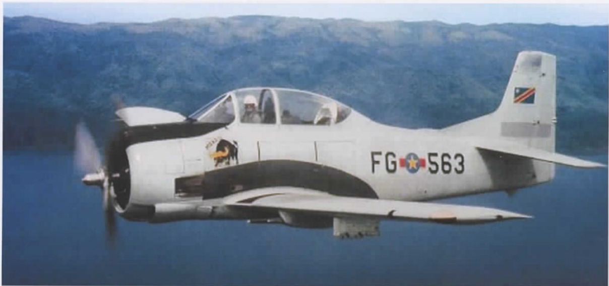
Above: FG-563 was one of the initial three T-28Ds delivered to the Congo. All were of the T-28D-5 version, with ammunition storage inside the wing. Unlike the T-28Bs and 'Cs, most of the T-28Ds were finished in overall USAF Gray. The aircraft is seen over Lake Tanganyika and carries the final, large version of the "Makasi" badge. Note the crudely over-painted USAF serial. (Terry Peet)
