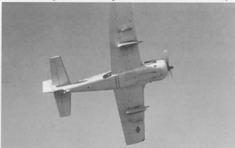
Rare view of the underside of one of the FAC T-28Cs, showing the speed brake to good effect. Aircraft FA-477 was one of the few to carry national insignia on the wings. (Luis de la Guardia)
