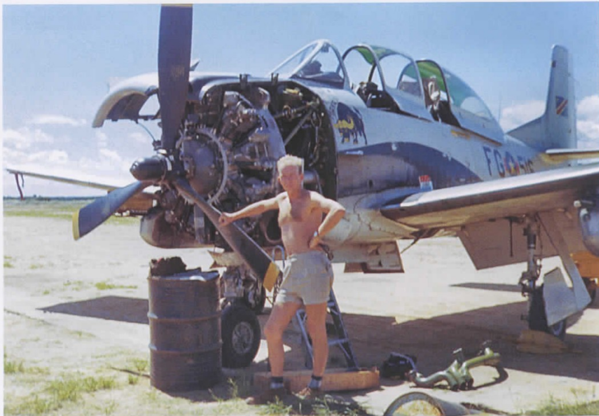
A WIGMO mechanic carries out field maintenance of a T-28C in 1966. The removed cowling provides a good view of the engine installation. (Dick De Boer)
