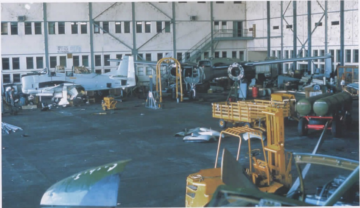
Above: A cluttered scene from the WIGMO hangar at N'Djili airport in May 1965, as one of the new T-28Bs (BuNo 138153) is being readied for operations. Behind it, a B-26B is being dismantled for parts. (Jan Hekker)
